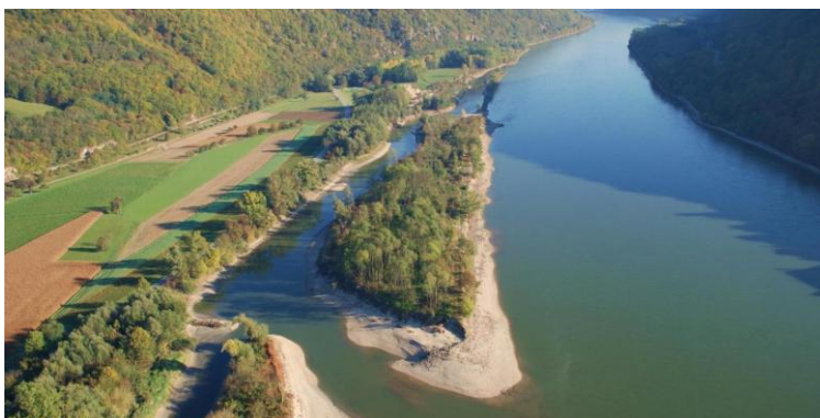
Top and below: The reconnected Schallengersdorf-Grimsing side-arm system after removing bank protection (riprap) and low-water regulation barriers © Haslinger, Seehofer
