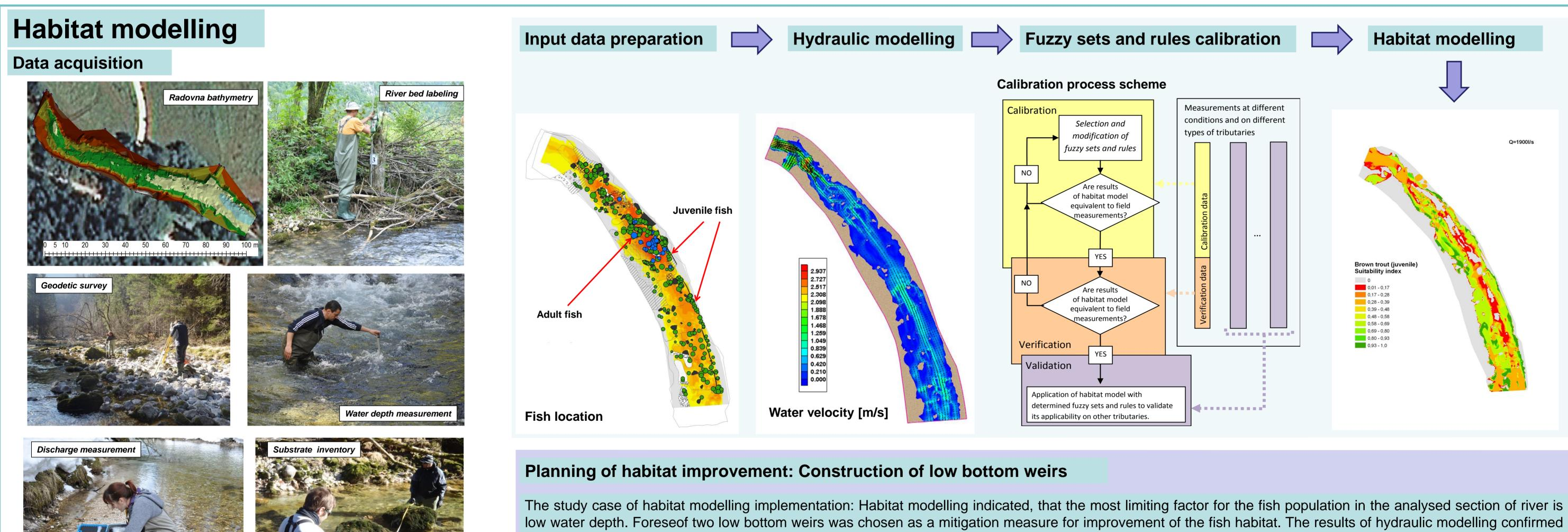
low water depth. Foreseof two low bottom weirs was chosen as a mitigation measure for improvement of the fish habitat. The results of hydraulic modelling confirmed higher water depth upstream of the weirs. Consequently, the habitat modelling results indicate improvement of fish habitat by the increase of weighted usable area (WUA) for juvenile and adult fish.
