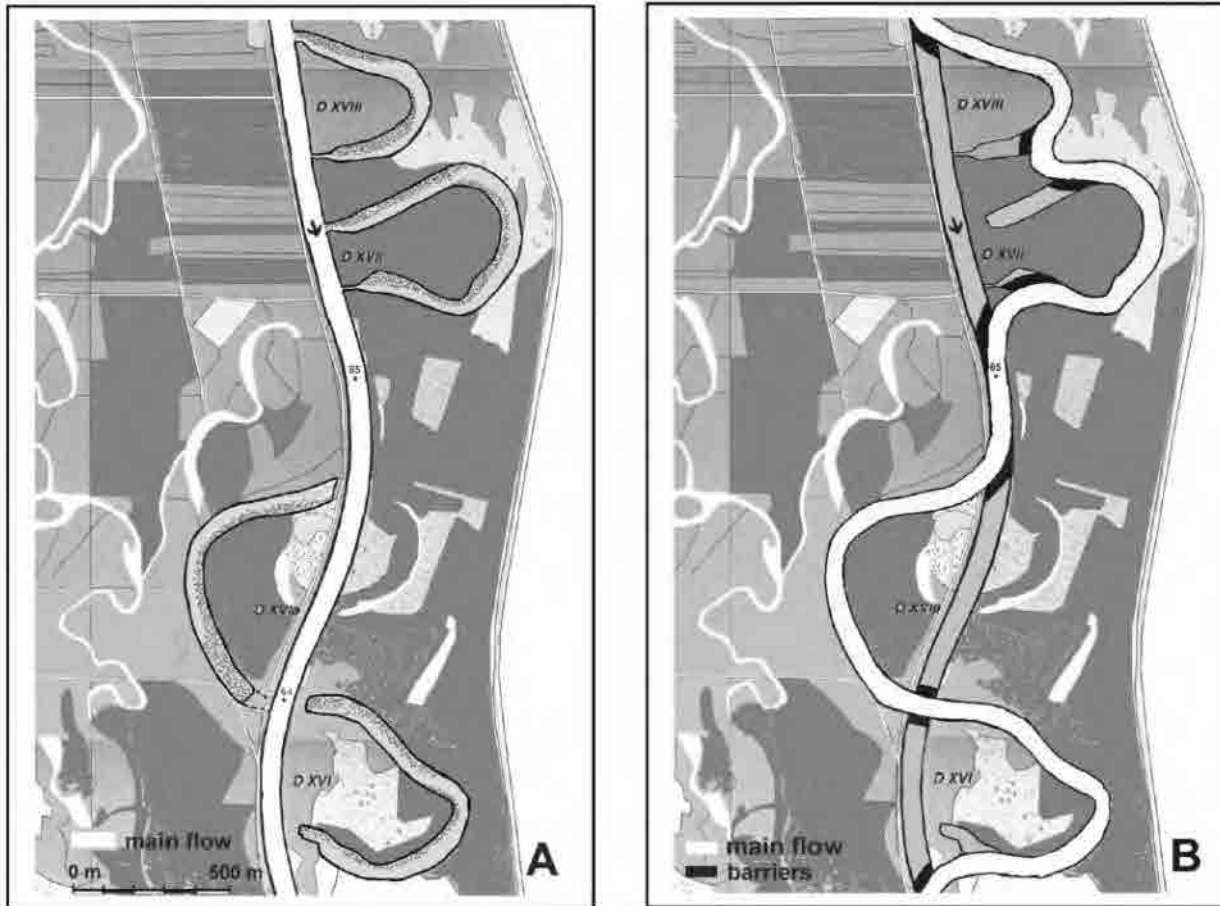
Fig. 2. Meander reconnection on the Morava river. A: present state; B: full meander integration (HOLUBOVÁ 2002).
