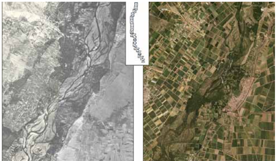
Comparison between orthophotos of a 5 km stretch of the Órbigo River taken in 1956 and 2006. They show perfectly the encroachment on the original channels, the channelization and the drastic morphological changes occurred in 50 years.
