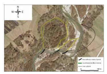
Czarny Dunajec River. Environment-friendly solution to the erosion threat to the local road, performed in the autumn 2011. Inlets to blocked braids distant from the road were opened and gravelly flow deflectors were formed in the main channel to direct flow to the re-activated braids.
