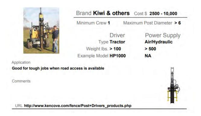
Figure 24 – Hydraulic drivers are available for mounting on skid steers, tractors, backhoes, excavators and mini-excavators. Here's one example from Kencove. We are not endorsing any specific band or manufacturers, but provide these for informational purposes only as these are readily available and have been used extensively in low-tech restoration.
