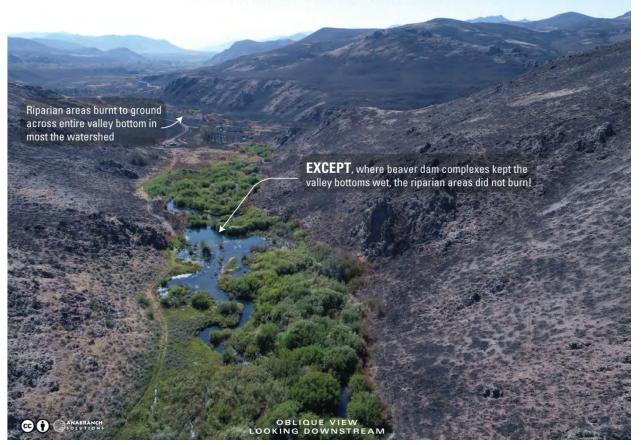
Figure 6 – Example of structurally-forced resilience to fire where beaver dam activity kept parts of the riverscape from burning, providing critical wildlife and livestock refugia during the fire, and assisting in post-fire recovery. Example from Baugh Creek, Idaho.
