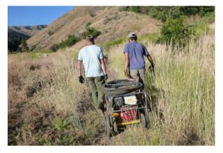
Figure 17 - Moving the power pack (Atlas LP 13-20) and hose that drives the hydraulic post driver is at least a two-person job if it can be rolled, and is often easier with three or four. It typically takes three to four people to lift and/or carry it short distances.
