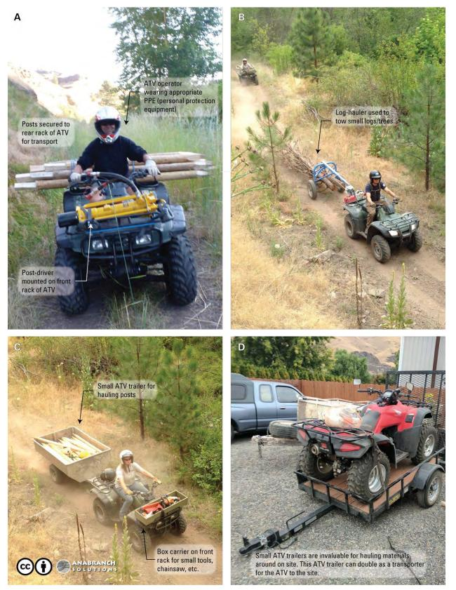
Figure 13 – Where ATV access is feasible, ATVs can be a very handy way of moving materials between staging areas and structure locations.
