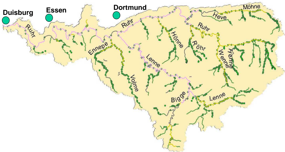
Fig. 1: Number and location of existing barrages within the Ruhr River Basin (in January 2003)
