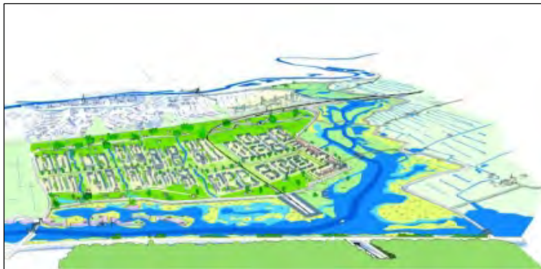
Figure 6 - Birdseye view of a bypass around the city of Kampen in the downstream part of the Rhine branch called the IJssel.
