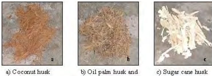
Figure 2 – Biological materials used to promote vegetation growth.
