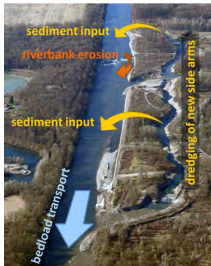
Figure 1 – Schematic drawing of the functionality of the measures.
