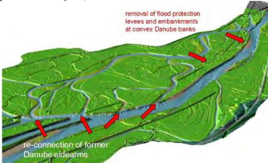
Figure 2 – As an example, model showing the maximum reconnection (restoration of surface connectivity) for the area based on historical analyses.
