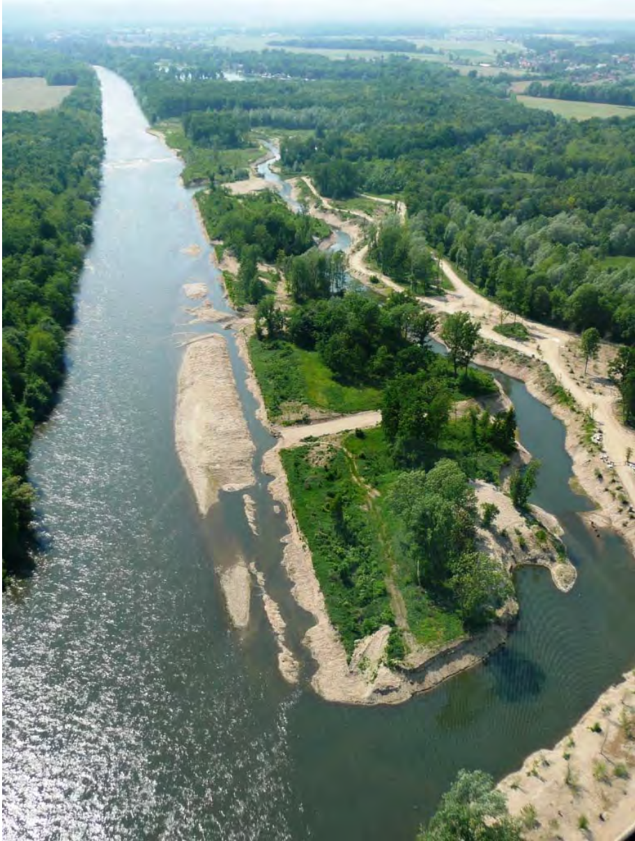
Figure 2 – Widening of the river bed in the Gosdorf area.
