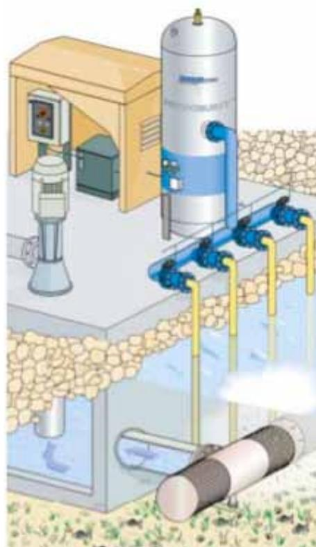
Protecting eels and other fish species from entrainment by installation of a suitable screen on water intakes
