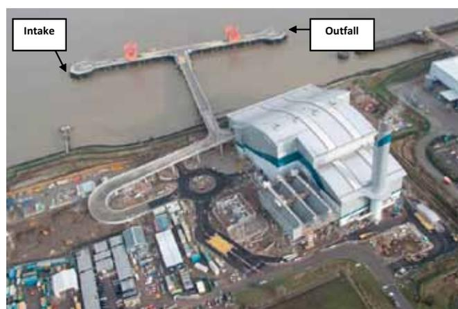
Energy from Waste Facility at Belvedere, with water intakes highlighted
