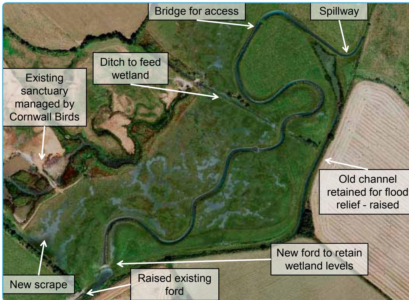
Plan indicating the location of the works. New wetland habitat in relic channels shown using LiDAR imagery
