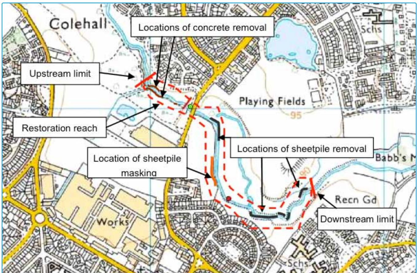
Schematic of the restoration works along the River Cole through Shard End
