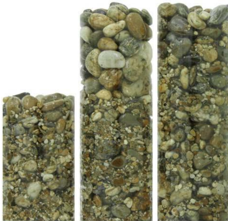
Figure 3. Gravel addition evolution: before, after (~25 cm of gravel addition) and final situation.
