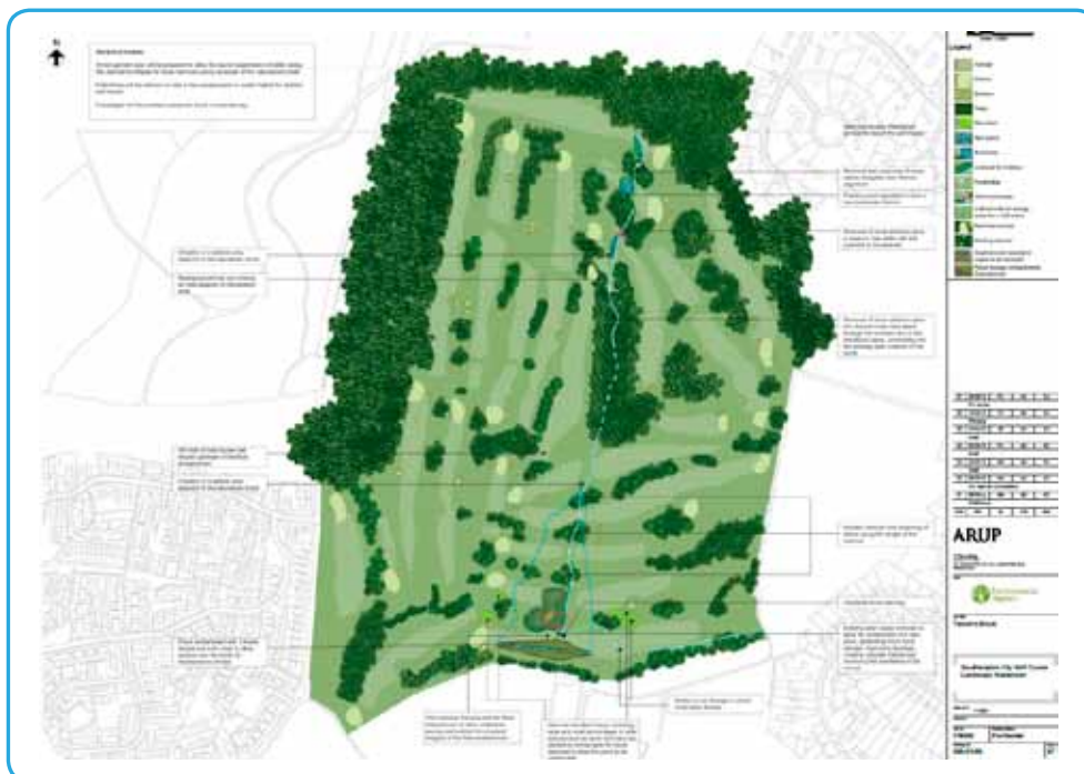
Holly Brook deculverting design
